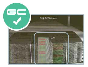
ERRORS DETECTED Gaps out of preset tolerance
